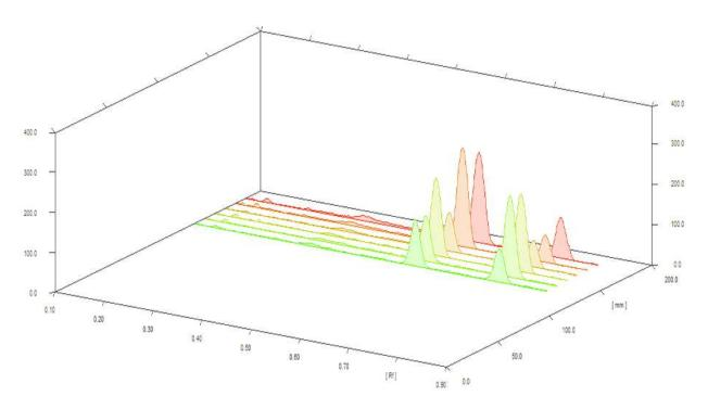
**Fig. 6.** six laboratory-prepared mixtures that were prepared with different ratios of TAMS and DUTA along with their linearity ranges at 270 nm
