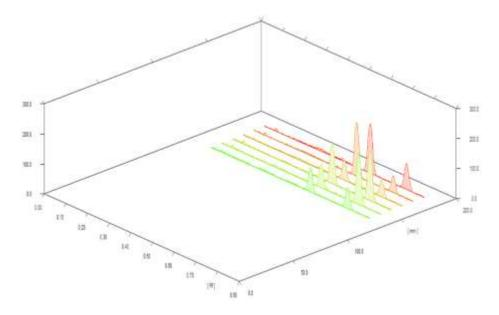
**Fig. 2.** Three dimensions TLC chromatogram showing the separation of TAMS ( $0.4 - 1.5 \mu g / spot$ ) from DUTA ( $0.5 - 1.5 \mu g / spot$ ) at RF =  $0.57 \pm 0.01$  and  $0.72 \pm 0.01$ , respectively at 270 nm
