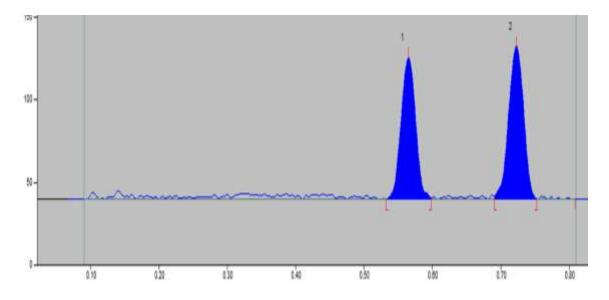
Fig. 3. Two dimensions TLC chromatogram showing the separation of TAMS ( $0.9 \ \mu g$  / spot) from DUTA ( $1 \ \mu g$  / spot) at Rf =  $0.57 \pm 0.01$  and  $0.72 \pm 0.01$ , respectively at 270 nm
