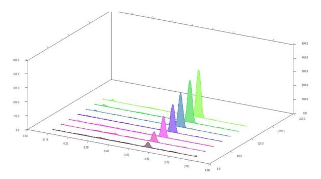
Fig. 4. Three dimensions TLC chromatogram showing TAMS linearity range (0.2 - 4  $\mu$ g / spot) at Rf = 0.57 $\pm$  0.01 at 270 nm
