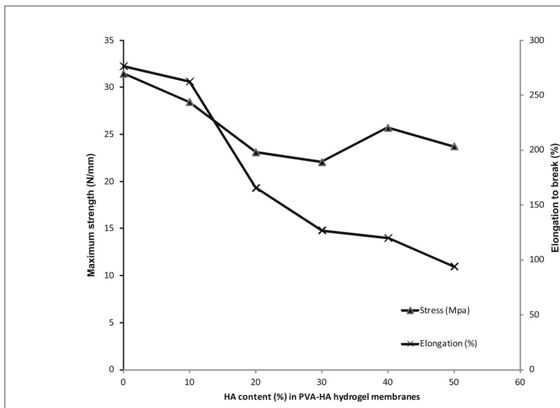
**Fig. 2-** Effect of hyaluronic acid content on mechanical properties of PVA hydrogel membrane.
