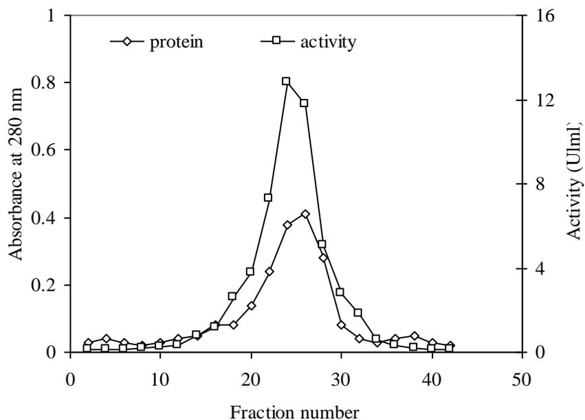
Figure (3). Gel filtration for the chromatography of Amylase DEAE-cellulose fraction on Sephadex G-200 column
