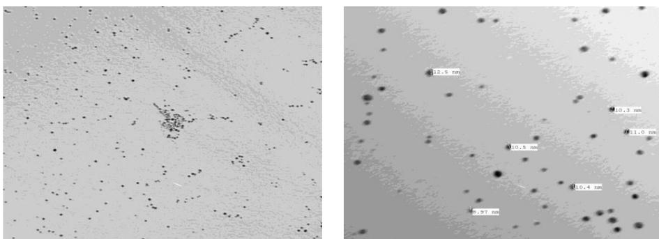
**Figure 1:** Transmission Electron Microscope (TEM) photos showing the particle size of gold nanoparticles (AUNPs).
