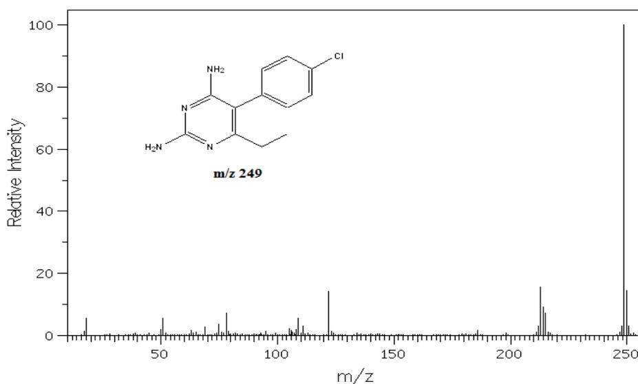
**Figure (3): Mass spectrum of pyrimethamine.**
