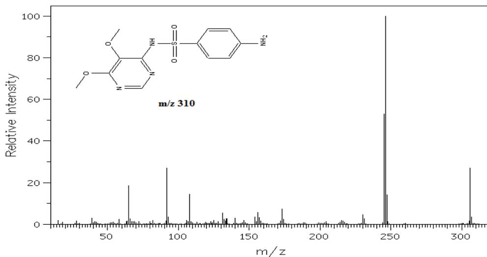
**Figure (5): Mass spectrum of sulfadoxine.**
