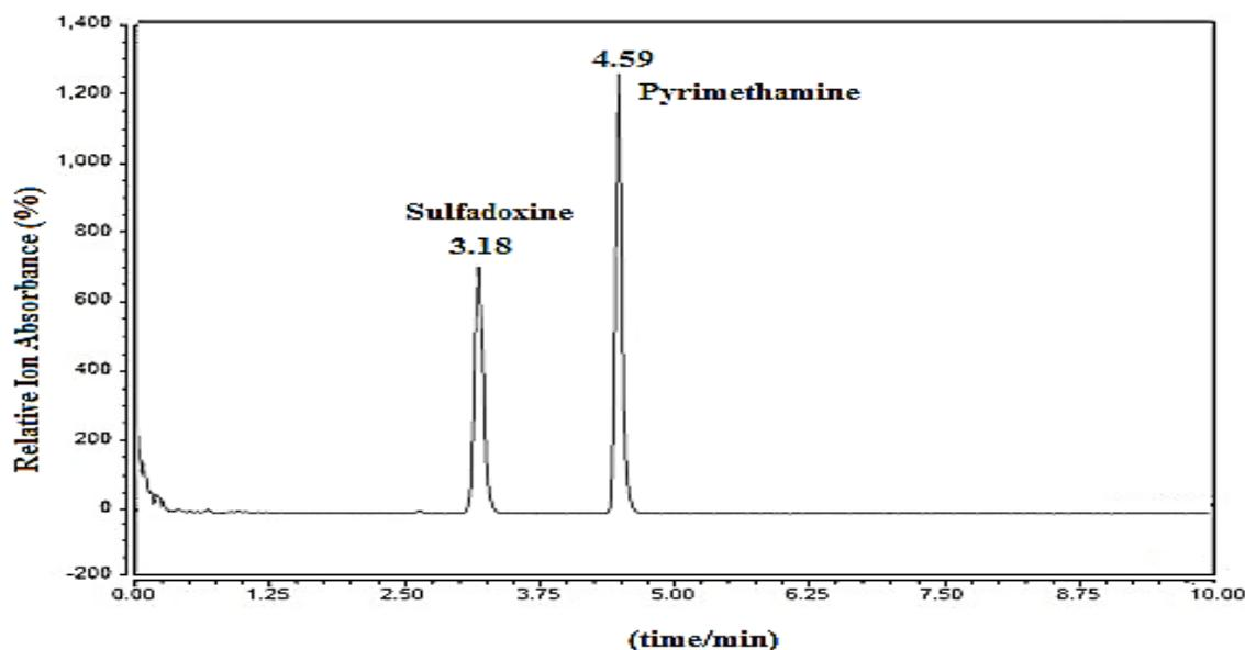
**Figure (2):** LC chromatogram of sulfadoxine (100 ng/ml) and pyrimethamine (20 ng/mL).
